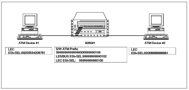
Figure 42. A Simple LANE Network - Physical View
